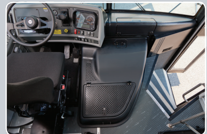
Engine access provides wider aisle for passenger loading and tool free access for serviceability.
